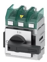
SENTRON, Molded case switch 3LD5 UL, Main switch, 3-pole, certified according to UL489 UL60947-4-1 and IEC60947-3, UL: 125A, SCCR 65kA at 480VAC, Operating power at 480VAC 3-phase: 75hp, IEC: 125A, Operating power at AC-23A at 400V: 55kW, floor mounting with direct handle, black, incl. terminal covers for the infeed side
