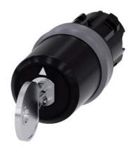
key-operated switch Siemens, 22 mm, round, plastic with metal front ring, lock number SSG10, with 2 keys, 3 switch positions I-O-II, latching, actuating angle  $2x45^\circ,\,10:30h/12h/13:30h,\,key\,removal\,O$
