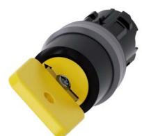
Key-operated switch O.M.R, 22 mm, round, plastic with metal front ring, lock number 73033, yellow, with 2 keys, 2 switch positions O-I, latching, actuating angle 90°, 10:30h/13:30h, key removal O+I, with laser labeling, inscription or symbol Customer-specific selection with SIRIUS ACT configurator (CIN)
