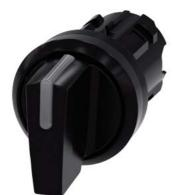
Illuminable selector switch, 22 mm, round, plastic, black, Selector switch short, 3 switch positions I>O<II, momentary contact on the left, latching on the right, actuating angle  $2x45^{\circ}$ , 10:30h/12h/13:30h
