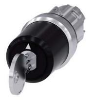
Key-operated switch BKS, 22 mm, round, metal, shiny, lock number S1, with 2 keys, 3 switch positions >0<II, momentary contact on the left, latching on the right, actuating angle  $2x45^\circ$ , 10:30h/12h/13:30h, key removal O, with laser labeling, upper case and lower case, always upper case at beginning of line
