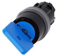
Key-operated switch O.M.R, 22 mm, round, plastic with metal front ring, lock number 73038, blue, with 2 keys, 2 switch positions O<I, momentary contact type, Actuating angle  $45^\circ,\,10:30h/12h,\,key\,removal$  O, with laser labeling, lower case
