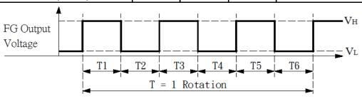
T= T1+T2+T3+T4+T5+T6=1 Rotation  $T = \frac{60}{rpm}$
