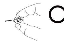
Don't pull fan with lead wires.
