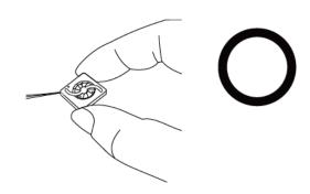
Don't pull fan with lead wires.
