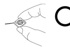
Don't pull fan with lead wires.
