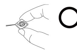
Don't pull fan with lead wires.
