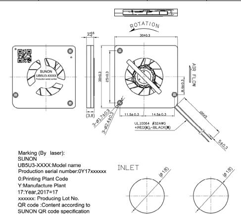
Sunon standard sample exclude the connector. If there is any request for connector, please advise in advance. About recommend connector, SUNON recommend the following models for SUNON Mighty Mini Fan/Blower: 1.(UST) SUR series connector: 02SUR-32S / 03SUR-32S / 04SUR-32S.
