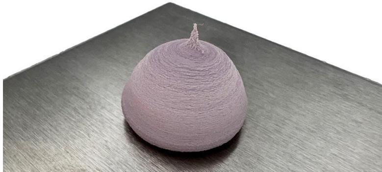
JONES Thermal Gel 21-361-SP02 is a soft, single part, silicone putty thermal gap filler in which no cure is required. This gap filler is designed to be used in where large gap tolerances are present and low mechanical stress on delicate components are needed. It is ideal for filling variable gaps between multiple components and a common heat sink.
