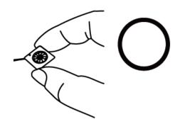
Don't pull fan with lead wires.
