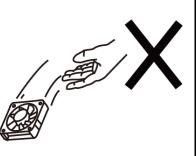
Don't cut the fan or lead wires
