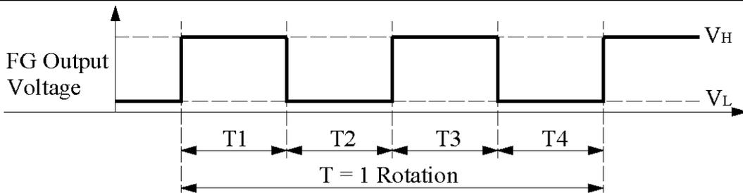
$T = T_1 + T_2 + T_3 + T_4 = 1 \text{ Rotation}$
