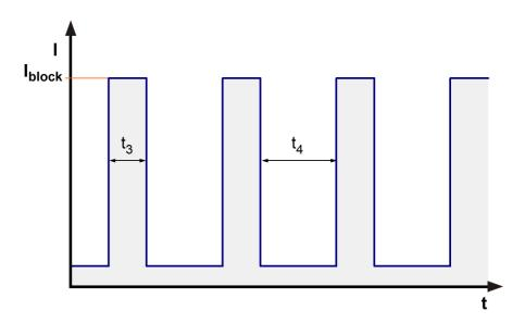
locked rotor current at 24V
