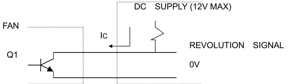
TRANSISTOR Q1 AT "ON" POSITION
