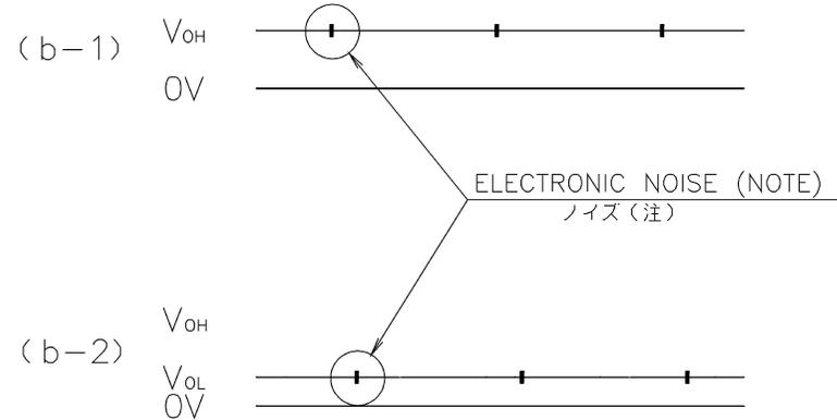
(NOTE) THE ELECTRONIC NOISE DUE TO AUTO-RESTART BEHAVIOR OF THE MOTOR
