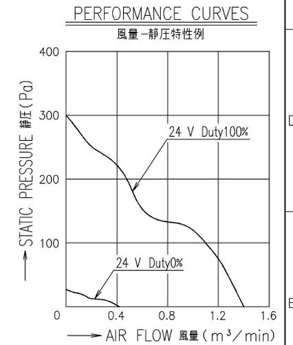
NOTE: 1. MEASURED AT 1 m DISTANCE FROM THE AIR INLET.
