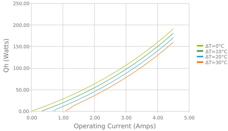
Total Heat Dissipated at Hot Side (Qh=Qc+Pin)
