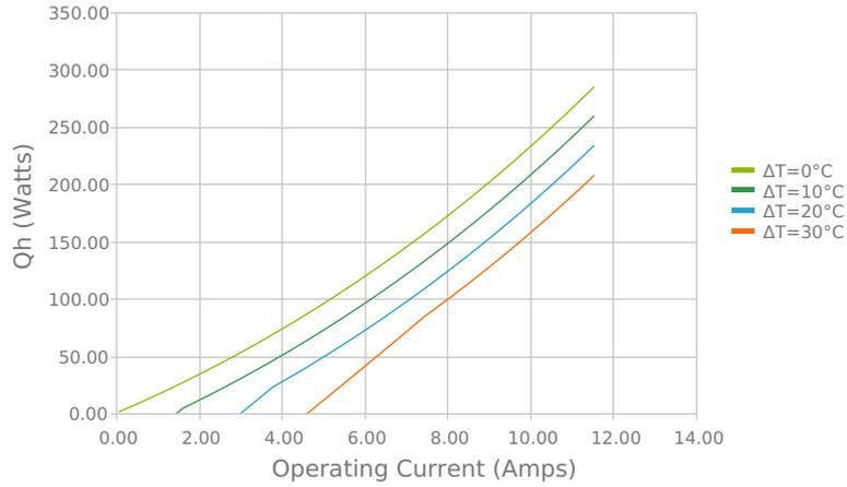
Total Heat Dissipated at Hot Side (Qh=Qc+Pin)
