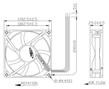
LEAD WIRES: UL 1007, AWG24, L = 290±10 mm Red = positive; Black = negative. White = FG
