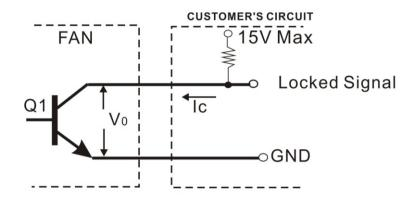
\*Transistor Q1 at "ON" position
