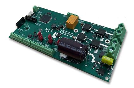
The Adaptive® JUNIOR is a PID controlled pulse width modulator (PWM), intended for thermoelectric cooler or heater applications that require a uni or a bidirectional drive source for accurate temperature control. The controller is capable of operating in a standalone mode, it is also supported by user-friendly PC software. There are additional quick set-up options for manual setpoint adjustment and a selectable fan voltage available.
