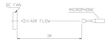
NOISE IS MEASURED AT RATED VOLTAGE IN FREE AIR IN SEMI-ANECHOIC CHAMBER WITH MICROPHONE AT A DISTANCE OF HALF METER FROM THE FAN INTAKE.
