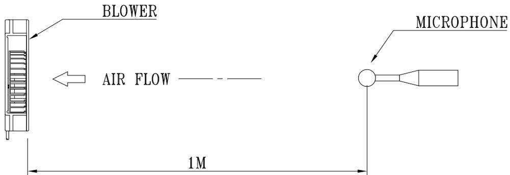
NOISE IS MEASURED AT RATED VOLTAGE IN FREE AIR IN ANECHOIC CHAMBER WITH B & K SOUND LEVEL METER WITH MICROPHONE AT A DISTANCE OF ONE METER FROM THE FAN INTAKE.
