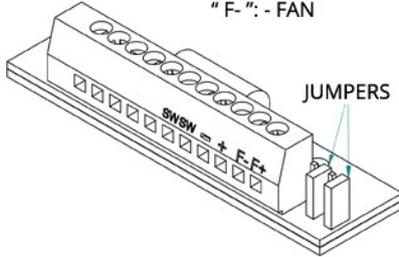
To use a separate supply for TEMs and FANs: Mount jumpers to not short-cut the pin pairs.
