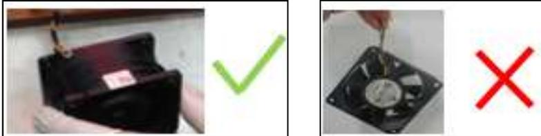
13-1-2. WEARING ELECTROSTATIC GLOVES BEFORE WORKING, MAKE SURE HOUSING ASSAMBLING MACHINE, WORKING TABLE WITH ELECTROSTATIC PROTECTION.
