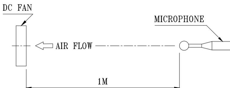
NOISE IS MEASURED AT RATED VOLTAGE IN FREE AIR IN ANECHOIC CHAMBER WITH B & K SOUND LEVEL METER WITH MICROPHONE AT A DISTANCE OF ONE METER FROM THE FAN INTAKE.
