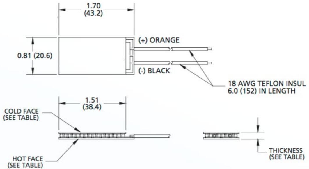
Ceramic Material: Alumina ( $\text{Al}_2\text{O}_3$ )
