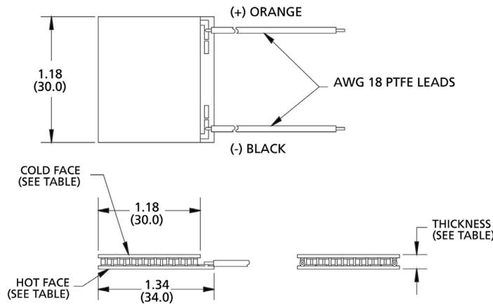
Ceramic Material: Alumina (Al<sub>2</sub>O<sub>3</sub>)
