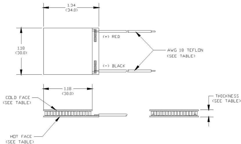
Ceramic Material: Alumina (Al<sub>2</sub>O<sub>3</sub>)
