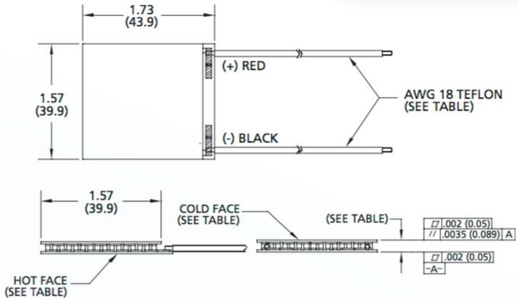
Ceramic Material: Alumina (Al<sub>2</sub>O<sub>3</sub>)
