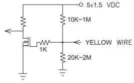
13-1. THE FAN SPEED WILL DEFAULT TO MAXIMUM WHEN THE SPEED CONTROL INPUT IS LEFT UNCONNECTED.
