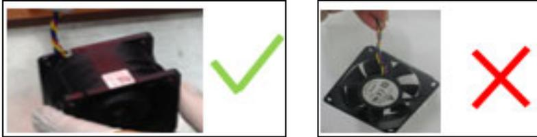
12-1-2. WEARING ELECTROSTATIC GLOVES BEFORE WORKING, MAKE SURE HOUSING ASSAMBLING MACHINE, WORKING TABLE WITH ELECTROSTATIC PROTECTION.
