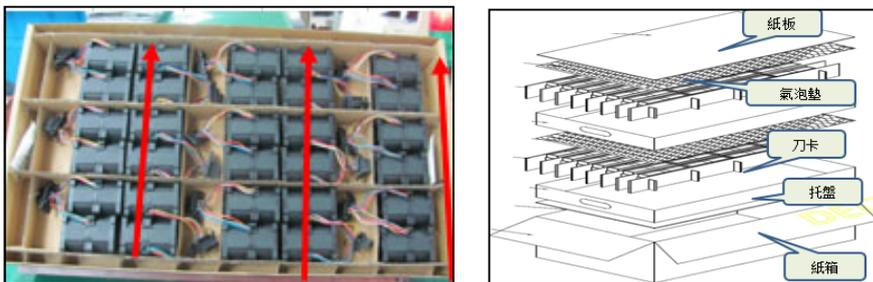
12-3-2. MAKE SURE DESICCANT, QUANTITY AND P/N IS CORRECT BEFORE PACKING.
