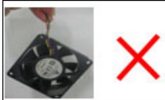
12-1-2. WEARING ELECTROSTATIC GLOVES BEFORE WORKING, MAKE SURE HOUSING ASSAMBLING MACHINE, WORKING TABLE WITH ELECTROSTATIC PROTECTION.
