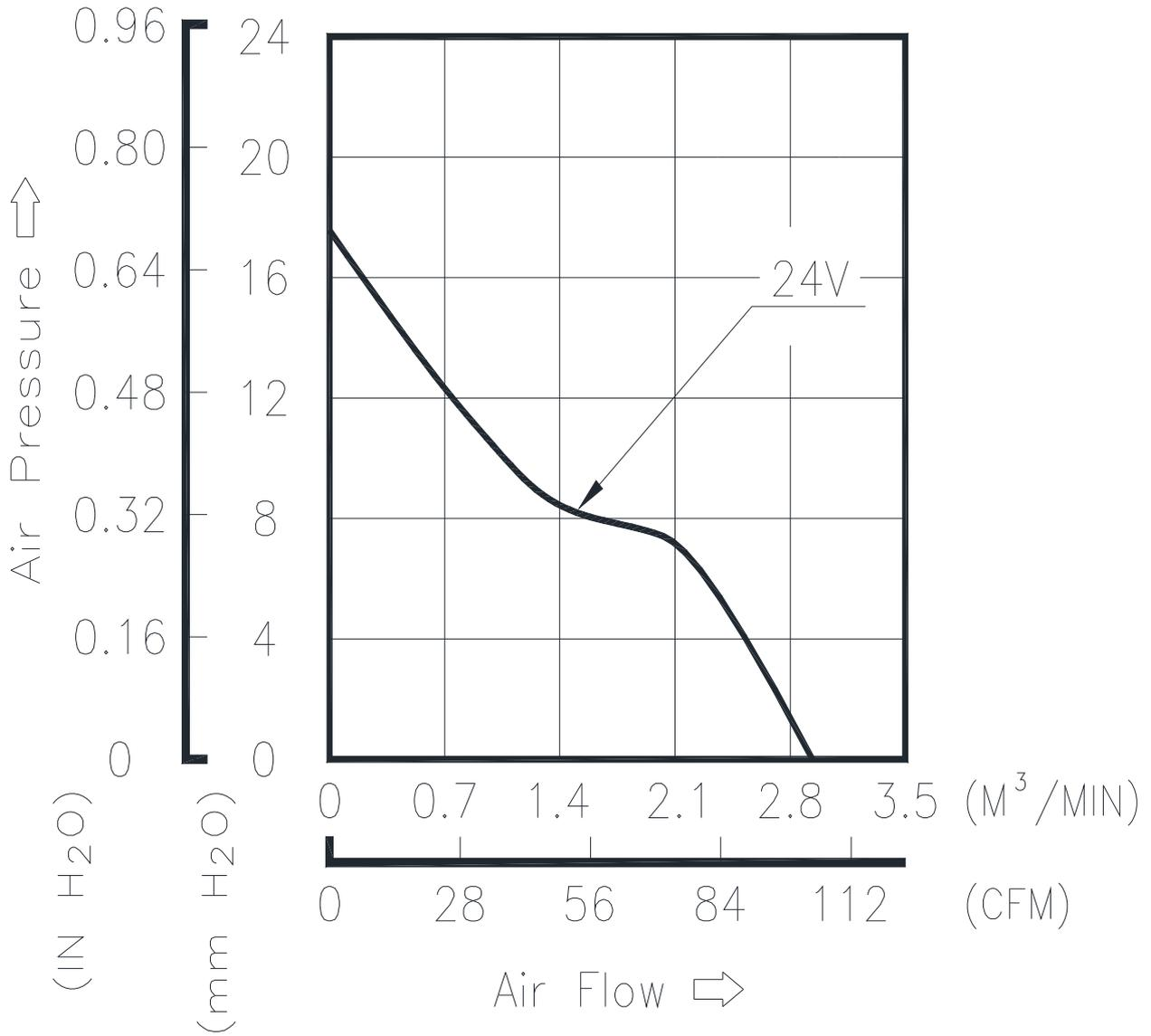
\*TEST CONDITION: INPUT VOLTAGE-----OPERATION VOLTAGE
