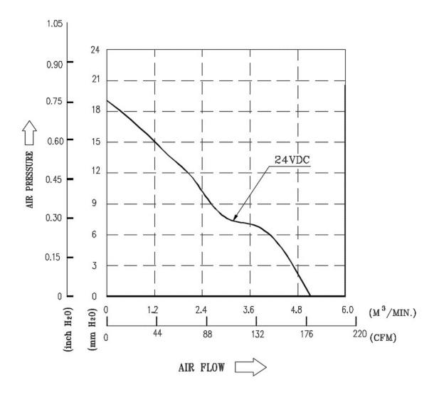
\*TEST CONDITION: INPUT VOLTAGE-----OPERATION VOLTAGE
