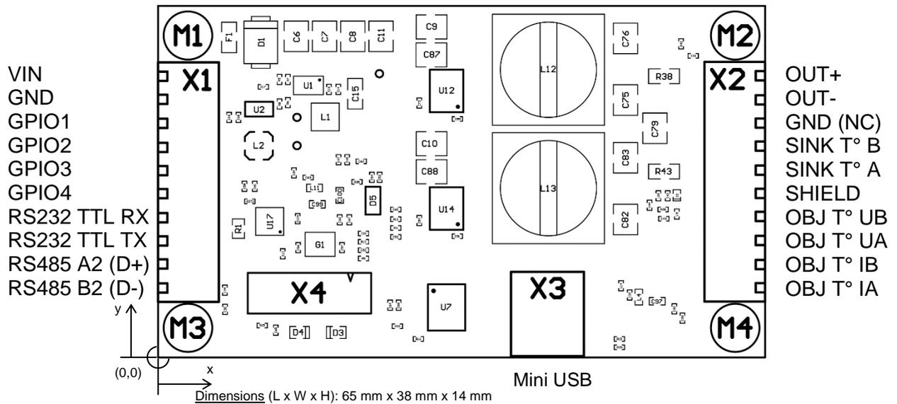
Figure 3: Package Outline and Pin Configuration of TEC-1091
