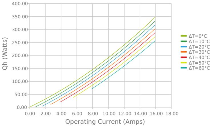
Total Heat Dissipated at Hot Side (Qh=Qc+Pin)
