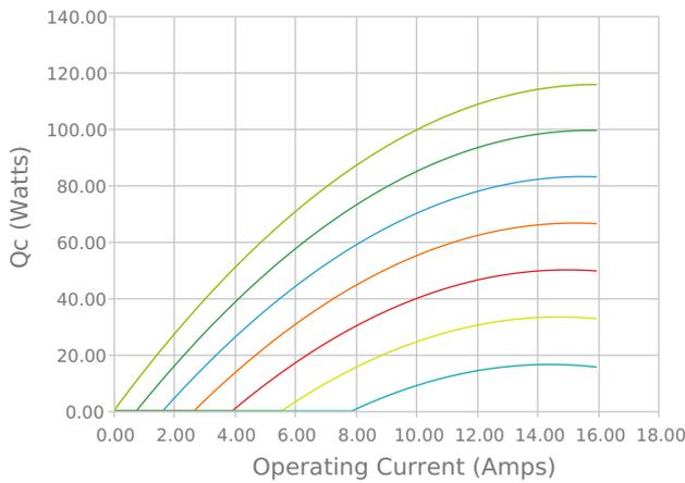
Heat Pumped at Cold Side
