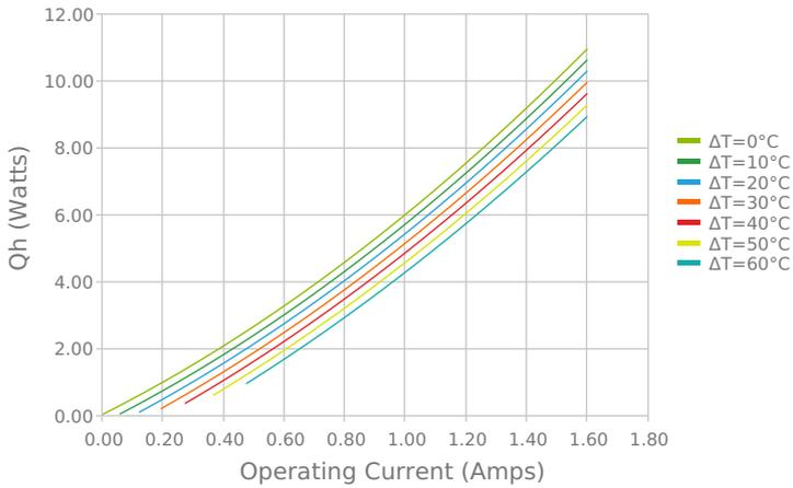
Total Heat Dissipated at Hot Side (Qh=Qc+Pin)
