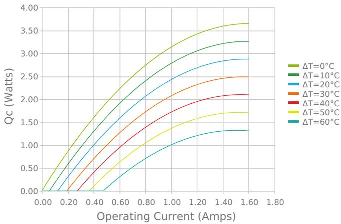
Heat Pumped at Cold Side
