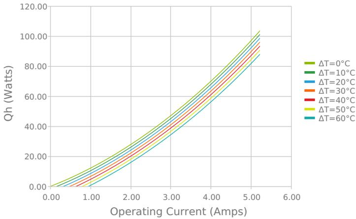
Total Heat Dissipated at Hot Side (Qh=Qc+Pin)
