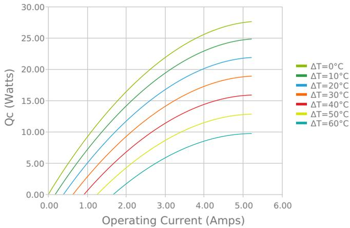
Heat Pumped at Cold Side
