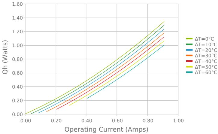
Total Heat Dissipated at Hot Side (Qh=Qc+Pin)
