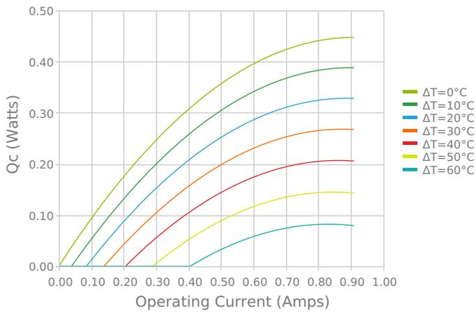
Heat Pumped at Cold Side
