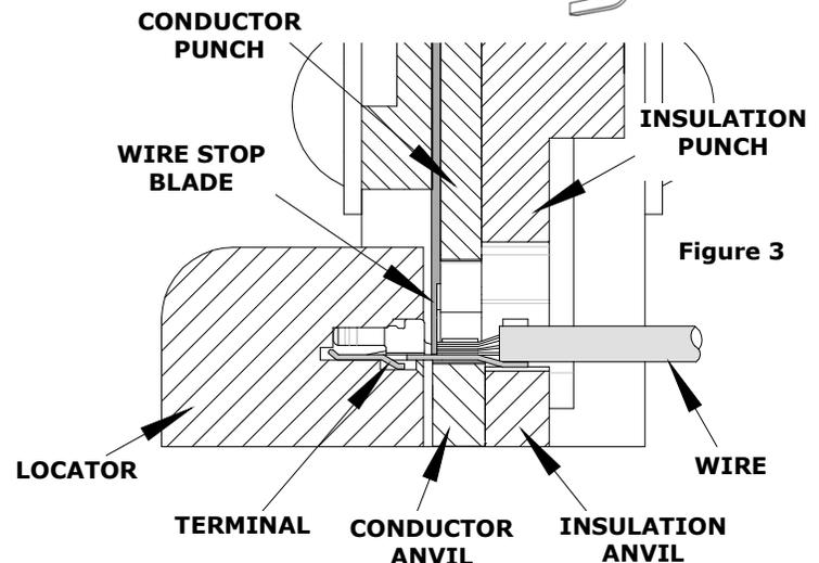
5. Slide the pre-stripped wire into the terminal, making sure to aim the wire brush toward the tip point on the wire stop blade. See Figure 2. Align the wire so that it is parallel and sitting into the terminal. Maintain a light and constant pressure on the wire that is seated in the terminal at all times. (Do not let go of the wire.) Be sure to hold the wire and terminal in place until the terminal is fully crimped. See Figure 3.
