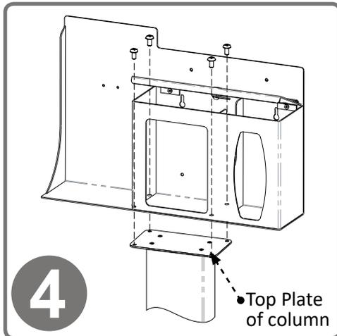
Attach the RS005-0212 Respiratory Hygiene Station to the column using (4x) screws included with stand. Tighten.
