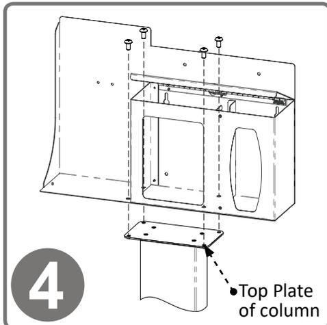
Attach the FD-062 Respiratory Hygiene Station to the column using (4x) screws included with stand. Tighten.
