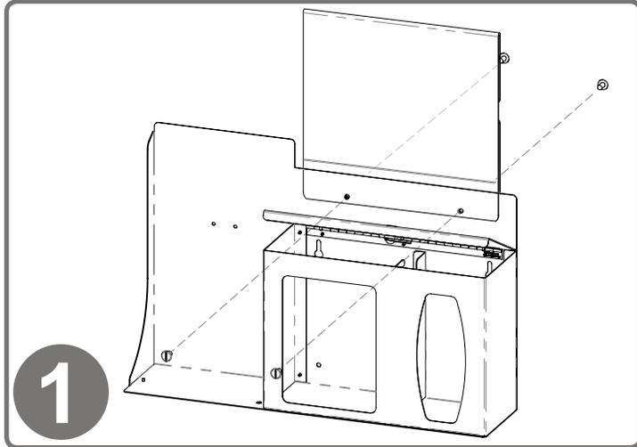
To mount the MP-075 Sign Holder, align the mounting holes of the holder with the holes on the top front of the dispenser. Attach using (2x) barrel screws included with sign holder.
