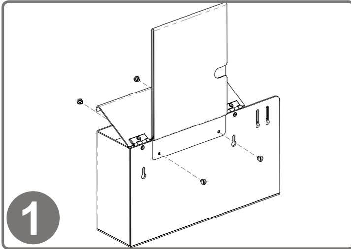
To mount the MP-070 Sign Holder, align the mounting holes of the holder with the holes on the top back of the dispenser. Attach using (2x) barrel screws included with sign holder.
