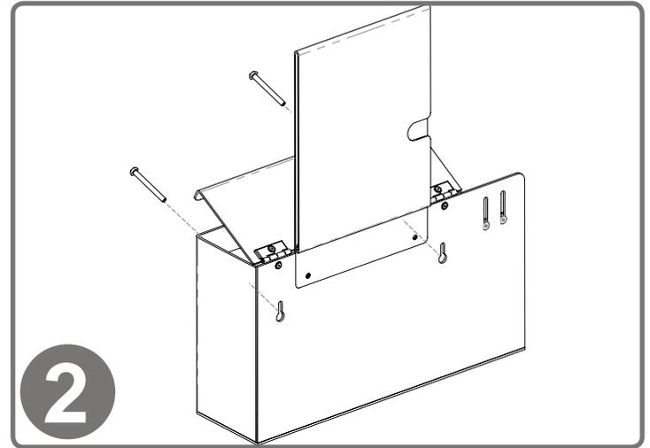
Dispenser can also be mounted securely to a wall through keyholes and screw holes in back with screws approved and supplied by building maintenance.
