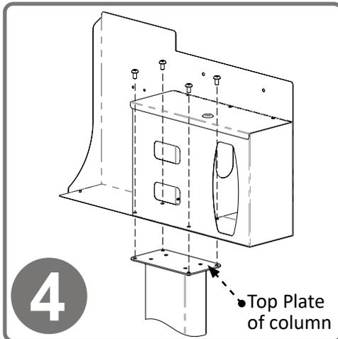
Attach the RS009-0420 Respiratory Hygiene Station to the column using (4x) screws included with stand. One pair of screw holes is located in the hand sanitizer dispenser section; the second pair are inside the facemask section and can be accessed with the lid open. Tighten all screws.
