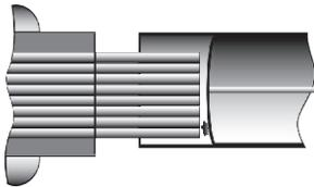
On the head of each CleanStixx™, fibres flex to easily conform to the end-face.
