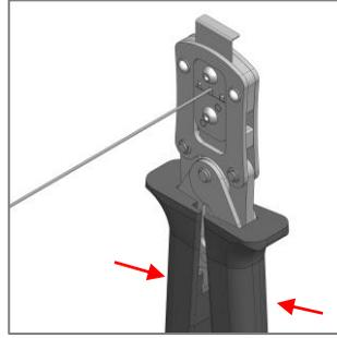
Insert the conductor up to the insulation stop plate
