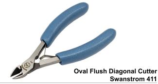
Body Width: .44 in Cutter Length: .38 in Overall Length: 4.875 in All-purpose cutter designed for use in general applications with a cutting capacity up to 16 gauge copper
