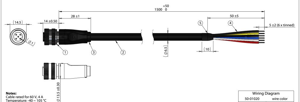
Notes: Cable rated for 60 V, 4 A Temperature: -40 ~ 105 °C Oil resistant up to 60 °C Water resistant up to 75 °C UV resistant
