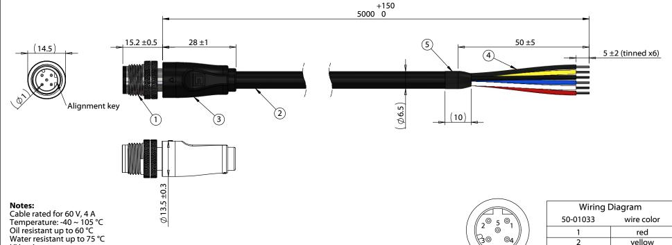
IP67 waterproof rating when mated with corresponding (IP67) connector
