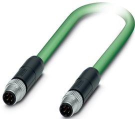
Network cable, PROFINET CAT5 (100 Mbps), EtherCAT® CAT5 (100 Mbps), 4-position, PUR/FRNC halogen-free, green RAL 6018, shielded (Advanced Shielding Technology), Plug straight M8 / IP67, coding: D, on Plug straight M8 / IP67, coding: D, cable length: 5 m
